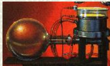
Expansion type cloud chamber
