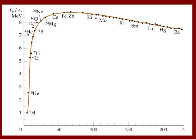
The fact that there is a peak in the binding energy curve in the region of stability near iron means that either the breakup of heavier nuclei (fission) or the combining of lighter nuclei (fusion) will yield nuclei which are more tightly bound (less mass per nucleon).
